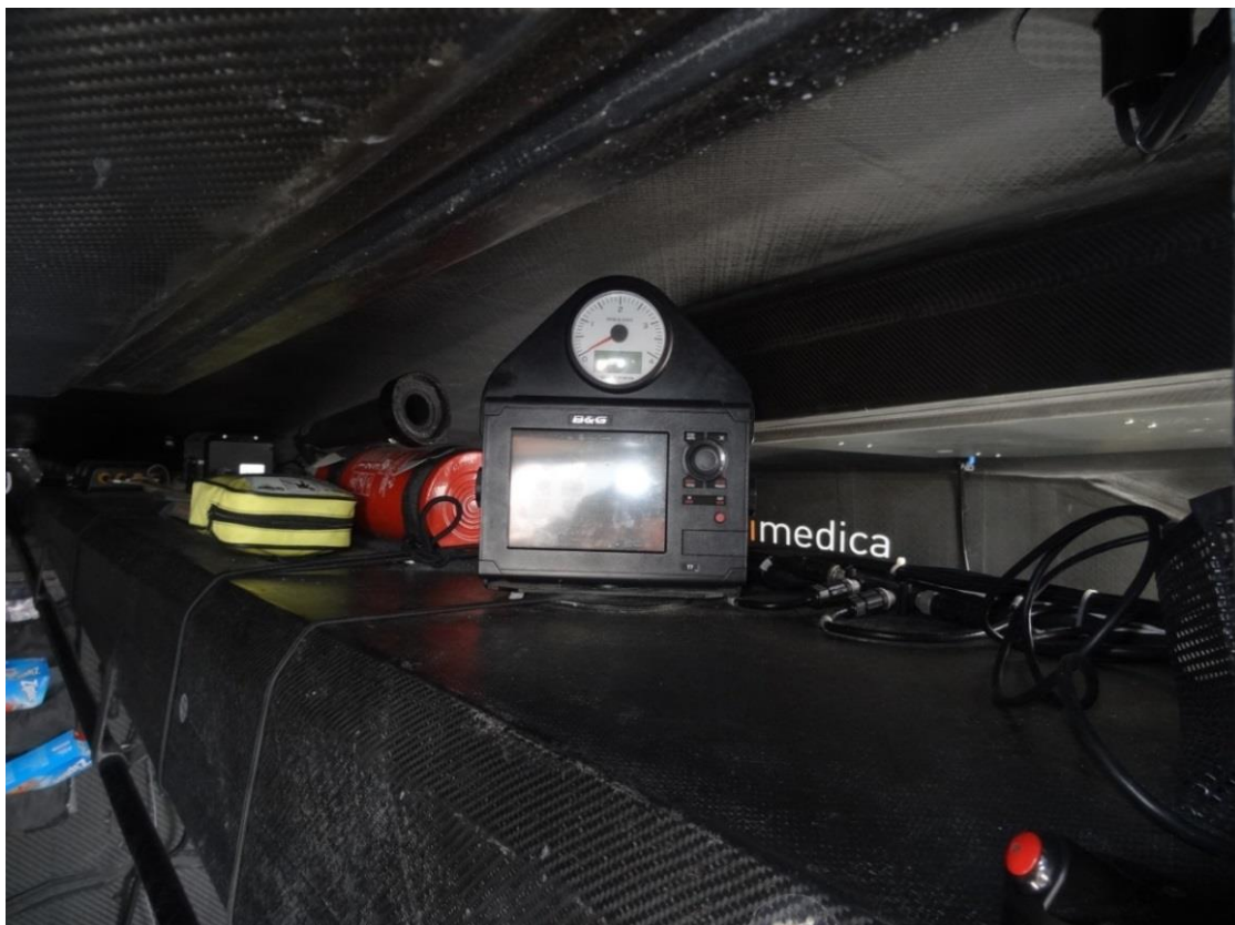
Figure 12 - Photo of the 'tunnel' MFD just inside the cabin available to crew on deck Credit: Photo by Chuck Hawley
