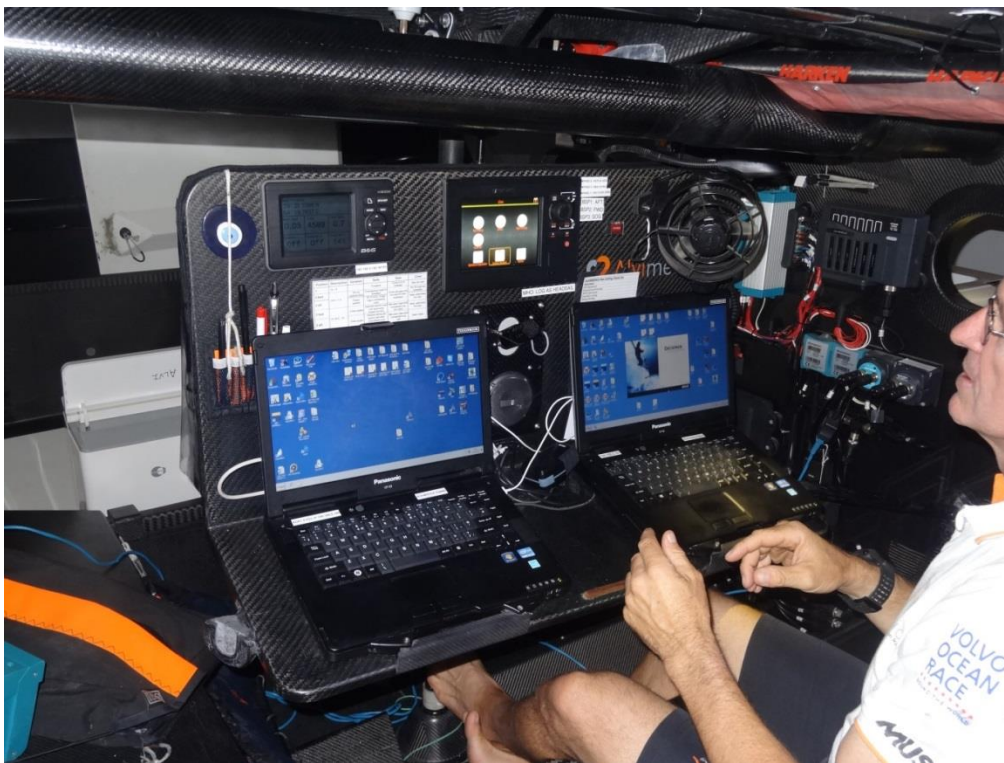
Figure 3 – Nav Station on board Alvimedica. A MFD display is located above and centred between the laptop screens. Nav station rotates on a vertical axis when boats are on the other tack.
