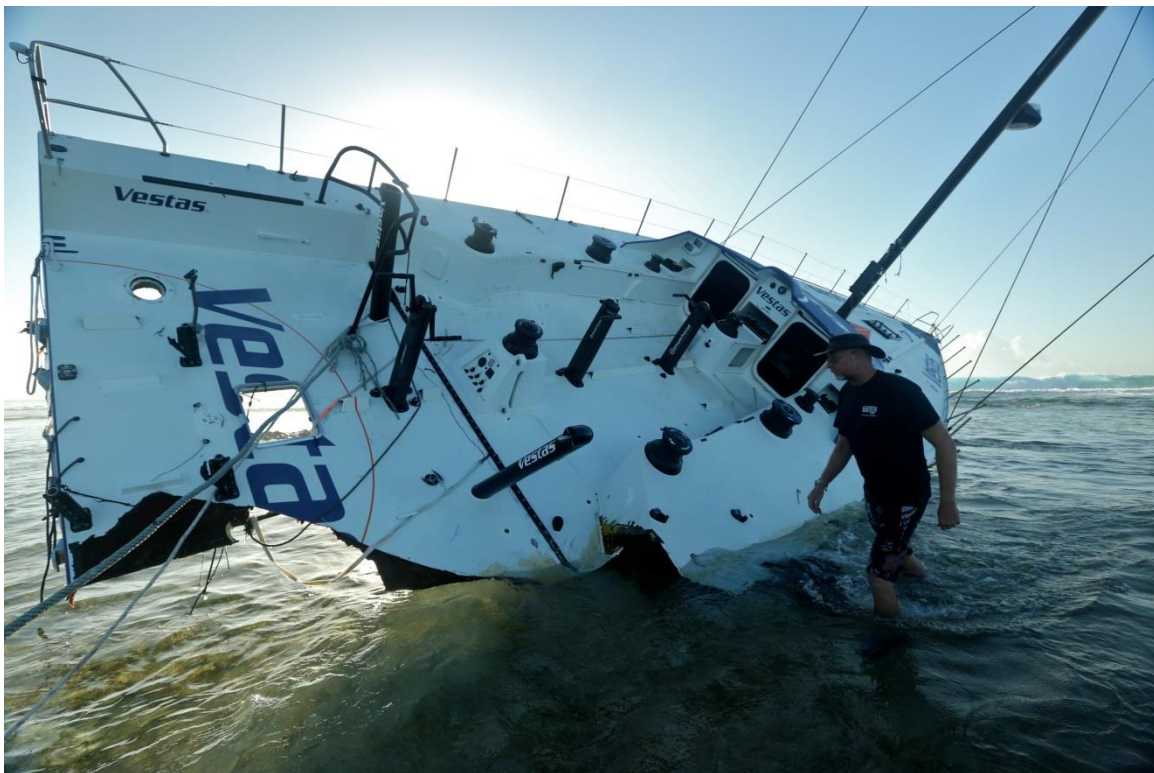
Figure 6 – A telling shot of the damage sustained to the starboard quarter Credit: Shane Smart/ Volvo Ocean Race
