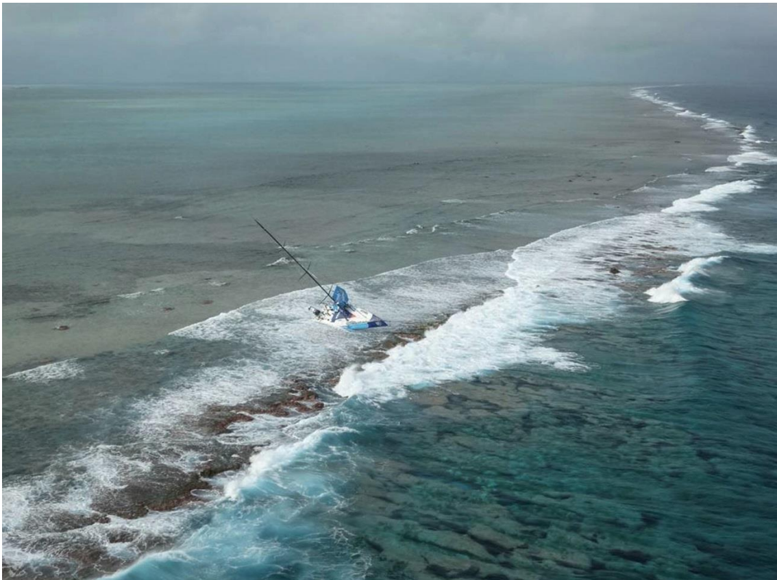
Figure 5 – The day after from the air – showing where the boat ended up, the reef face ahead of it with the breaking waves and the gutters in the seabed bottom where the keel was caught Credit: National Coast Guard of Mauritius
